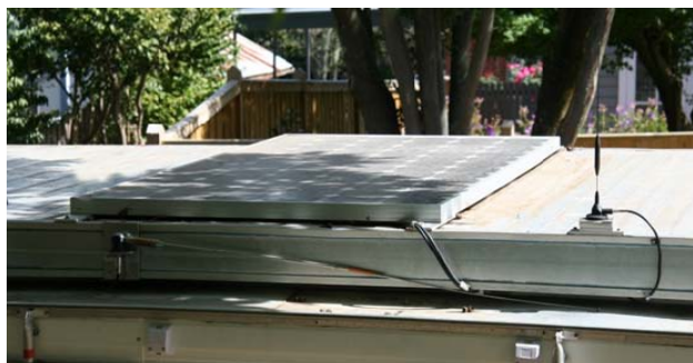
A 180w solar panel mounted on the roof of pop top caravan using aluminium brackets. This panel will be raised 30mm higher for better panel ventilation.
