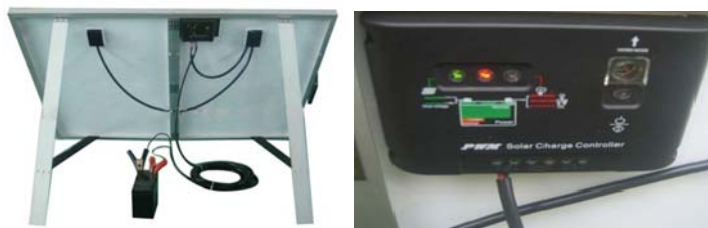
Fold out panel showing the panel, controller, battery and alligator clips
