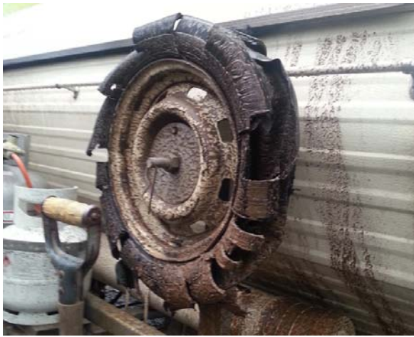
The remains of the shredded tyre. Have you checked yours recently?
